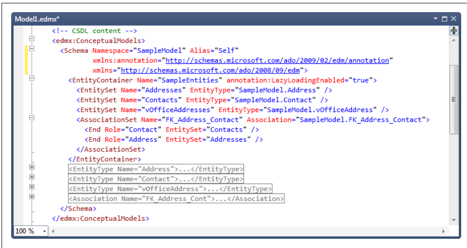
Figure 2-10. Expanding the conceptual model, its schema, and the EntityContainer inside the schema
